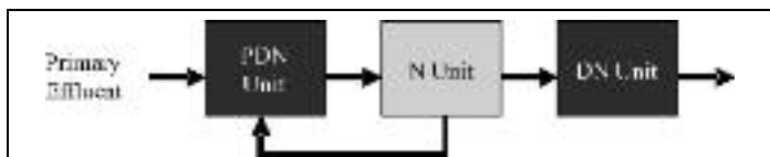
Figure 5. Three-stage pre-denitrification (PDN) process configuration
