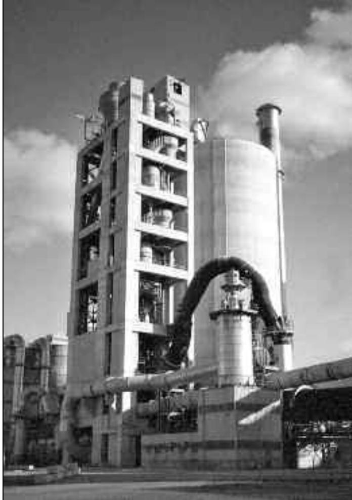
A cement kiln plant where mercury and its compounds can condense on the exhaust gas route due to cooling of the gas and are partially adsorbed by the raw material particles.
