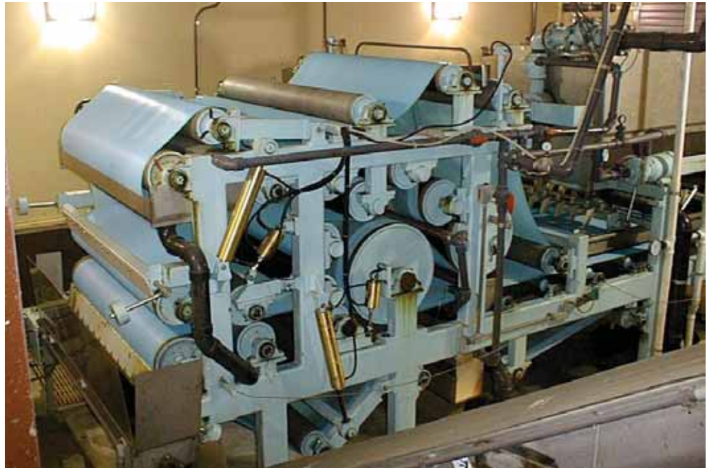
A belt press is often used to dewater sludge.
