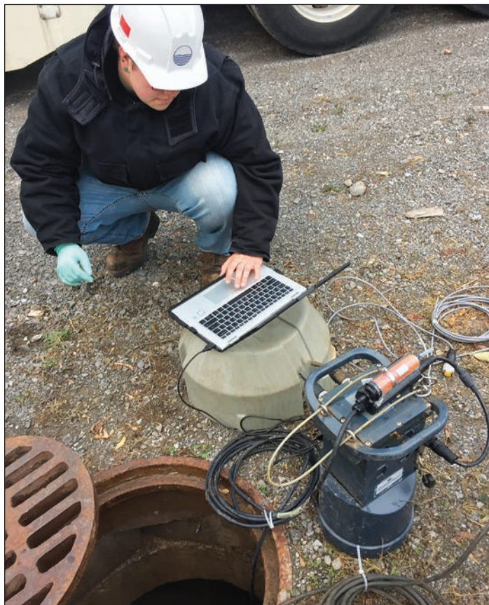
Monroe County field sampling crew conducts a flow monitoring study at an industrial site. MCDES
