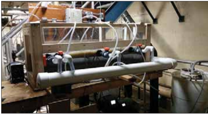
Nicknamed “Frank Jr.,” the pilot-scale aeration system is constructed and operated by the Van Lare WRRF staff. MCDES
