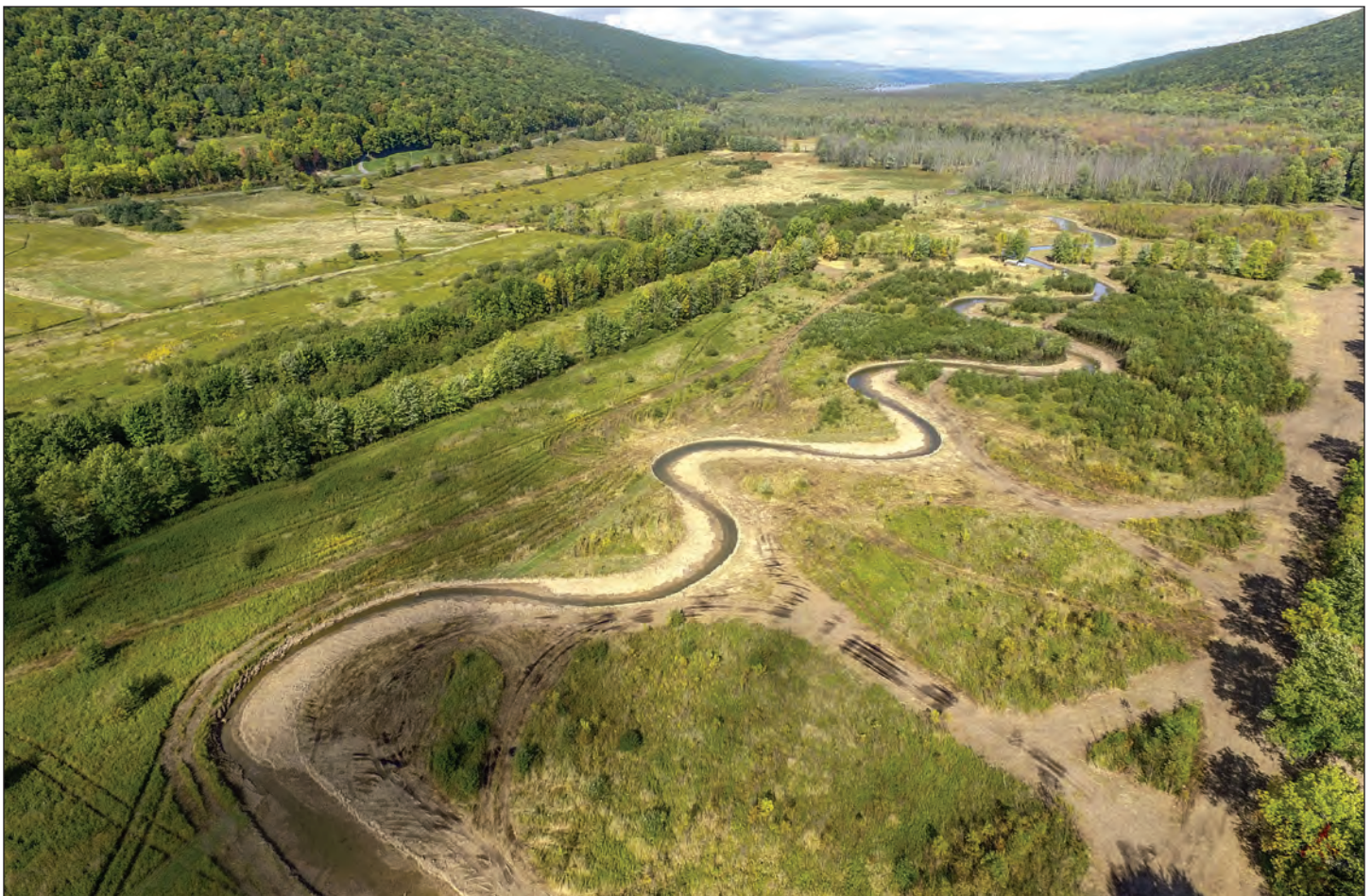
Honeoye Inlet and floodplain. This aerial view of the stream course, taken in October 2016, shows how it was restored into a winding channel that reconnects the Honeoye Inlet with its floodplain.
