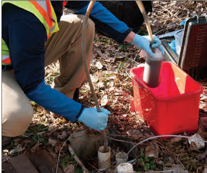
Groundwater sampling will be one component of the focused monitoring program to identify the source of bacterial contamination to the stream that discharges near Crescent Beach. istockphoto.com
