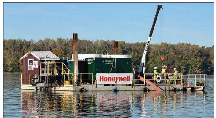
Figure 3. Nitrate addition barge on Onondaga Lake. Parsons
