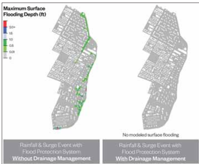
Figure 6. Sample two-dimensional modeling outputs indicate surface flooding benefits of drainage management for inland flooding during a coastal storm surge event. Hazen and Sawyer
