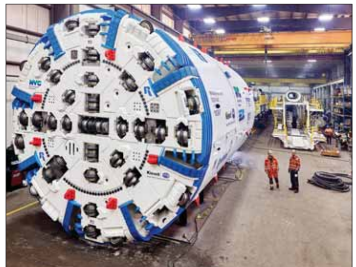
The unique tunnel boring machine (TBM) was named "Nora" and will be used to build a 14-foot diameter bypass tunnel to repair leaks in the Delaware Aqueduct. New York City DEP
