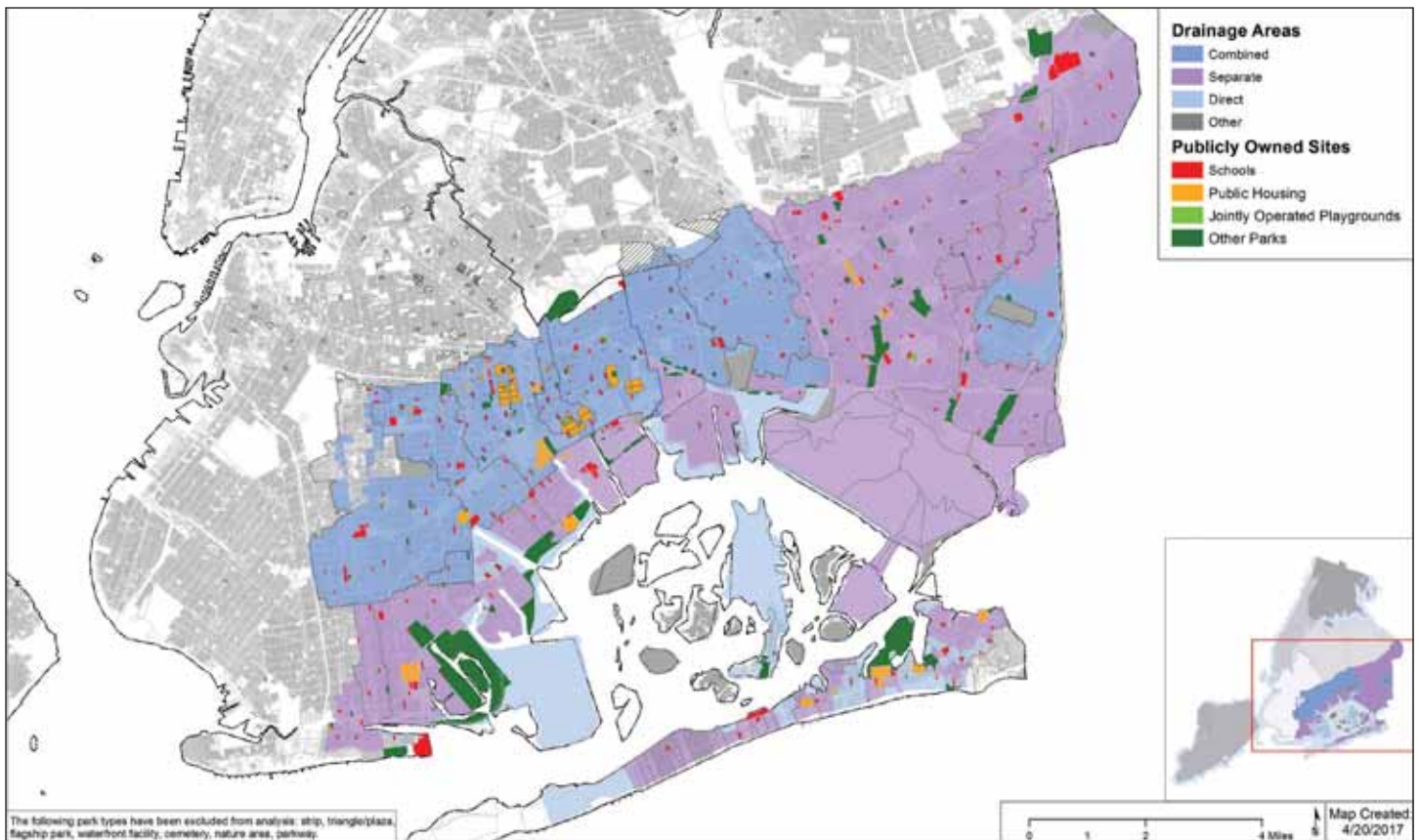
Figure 3. Integrated stormwater planning for public sites in the Jamaica Bay watershed involves managing different types of drainage areas.
