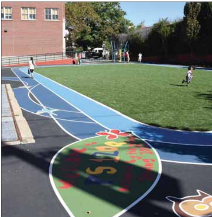
The playground at Public School 120 in Flushing, Queens, uses 3,500 crushed toilets below its surface to provide stormwater retention during rain events. New York City DEP
