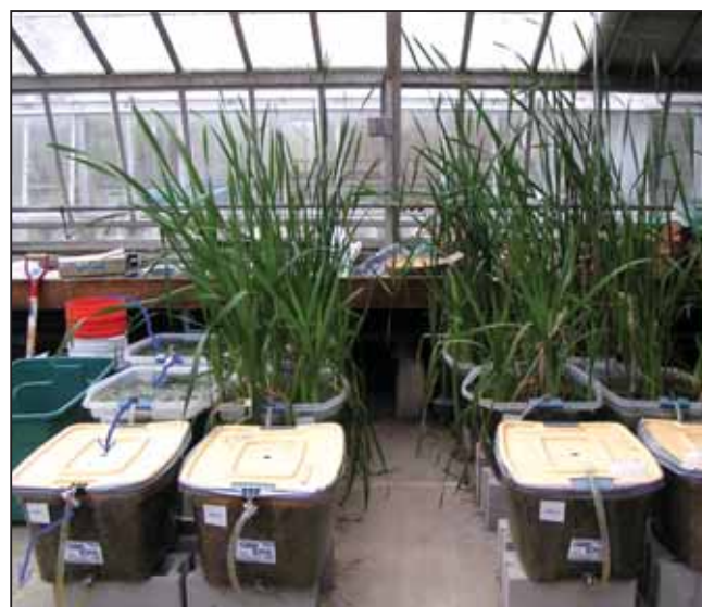
Figure 2. First generation of wetland treatment systems to initiate simultaneous nitrification, anammox and denitrification. Four systems were operated in parallel (from left to right) for treatment of ammonia-rich wastewater. Each system included two free water surface wetlands (back) and one biofilter packed with pea pebbles (front) in series. Six free water surface wetlands had broadleaf cattails.
