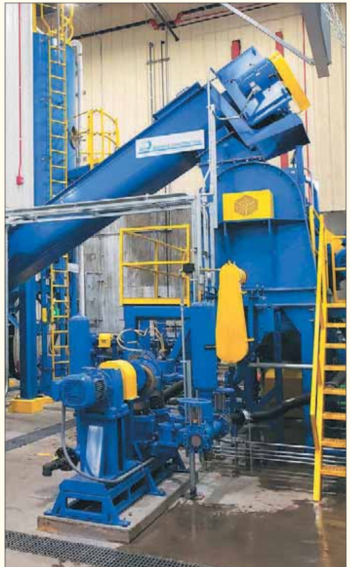
Depackager unit processing and separating packaging from food at OHSWA Food2Energy Facility. Emily Albright, OHSWA
