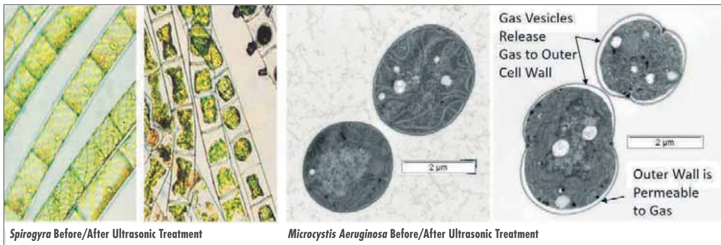
Figure 3. Spirogyra (left) and Microcystis aeruginosa (right) before and after ultrasonic treatment. Scanning electron microscopy of Microcystis aeruginosa was prepared by Dr. Paul Zimba of Texas A&M University, Corpus Christi. SonicSolutions Algae Control, LLC
