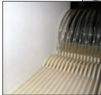
Figure 5B (left) is a close up showing the top of the SMU where several plates are mounted in parallel with hoses to withdraw clean filtered water out into a manifold that would connect to a permeate pump.
