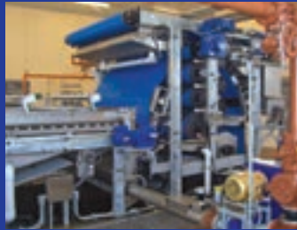
Dual Purpose 1.5 m model 3DP Operates as a GBT or Belt Press.
