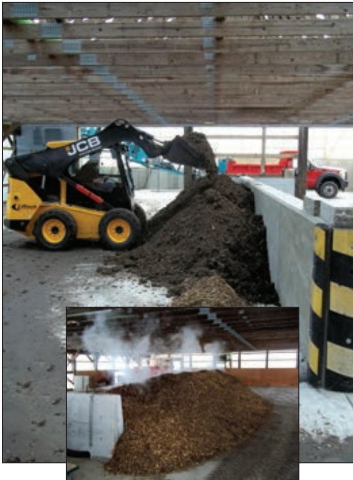
Piling the compost mix over the air line – called the static pile – for temperature, biological processing for 21 days; and the pile is shown when at temperature between 55–57 degrees Celsius.
