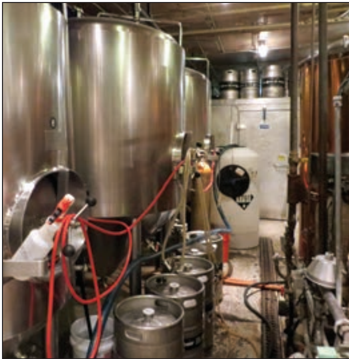
A New York brewery where beer fermentation tanks generate yeast wastewater and tests occur for organic loading to the wastewater system.
