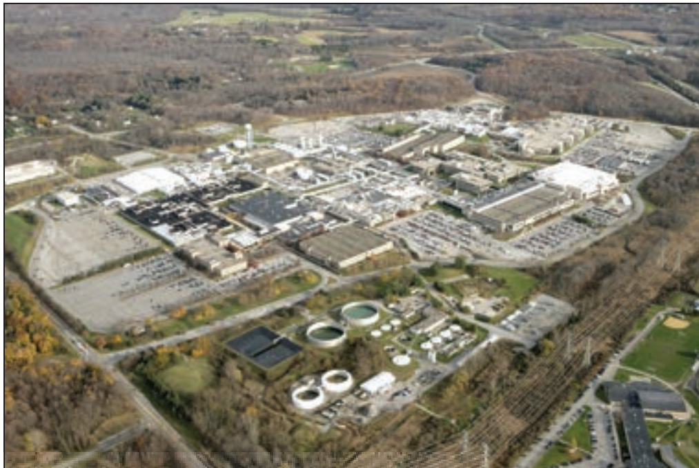
Aerial of IBM East Fishkill, NY site includes eight different treatment plants. The big tanks at bottom are the last point of treatment before discharge to the stream, Gildersleeve Brook.
