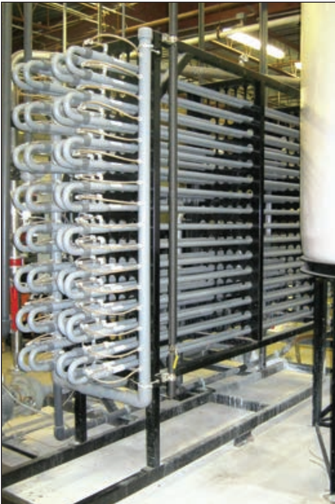
The ultrafilter unit's tubular membranes can process up to 6,000 gallons per day. On the right is the conical tank that feeds the ultrafiltration unit new and concentrated wastewater.
