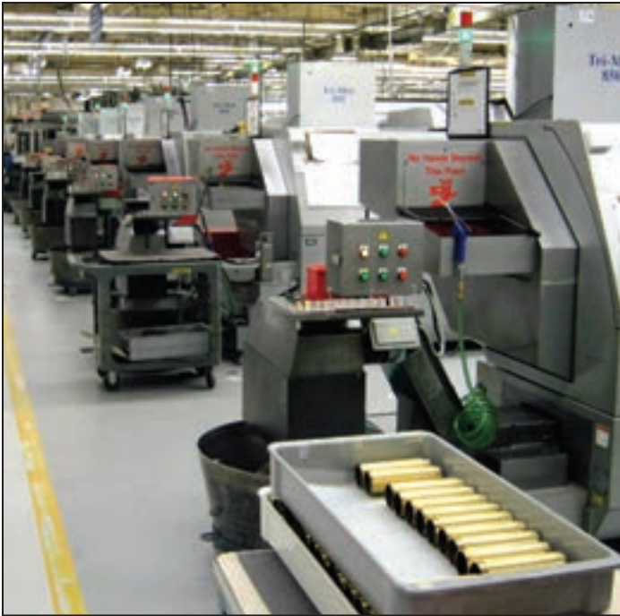
A row of CNC machines at the Welch Allyn facility used to fabricate brass parts (seen in foreground) for medical products. A change to vegetable-based oil used in the machining process unexpectedly led to higher hexane extractable residuals found in its wastewater.
