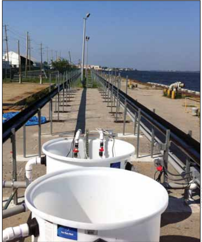
An algal turf scrubber was constructed at the Rockaway WWTP to test its efficiency at filtering out nutrients and potential for conversion of the algae to biofuel.
