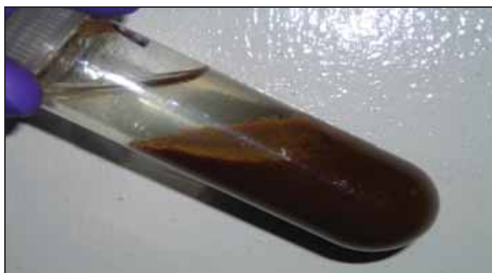
Separation of anammox granules using the centrifuge method. Performed under the mainstream deammonification lab-scale pilot tests at Blue Plains Advanced Wastewater Treatment Plant under INFR6R11 to promote research into low energy alternatives to conventional processes.
