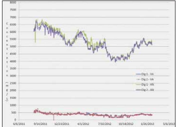
Figure 6. Levels of alkalinity and volatile acids in digesters 1 and 2.
