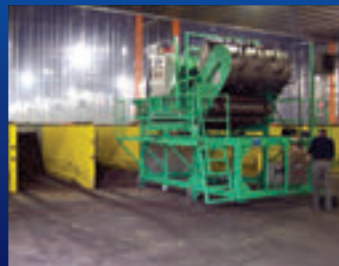
Agitated and Aerated In-vessel type Composting System (ICS)
