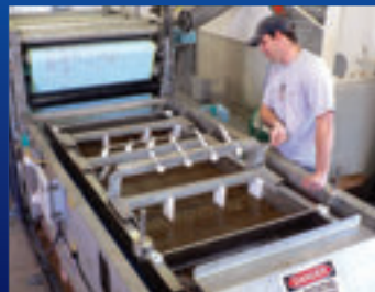
Compact 0.9 m Model DDP Belt Press Great concept for small plants
