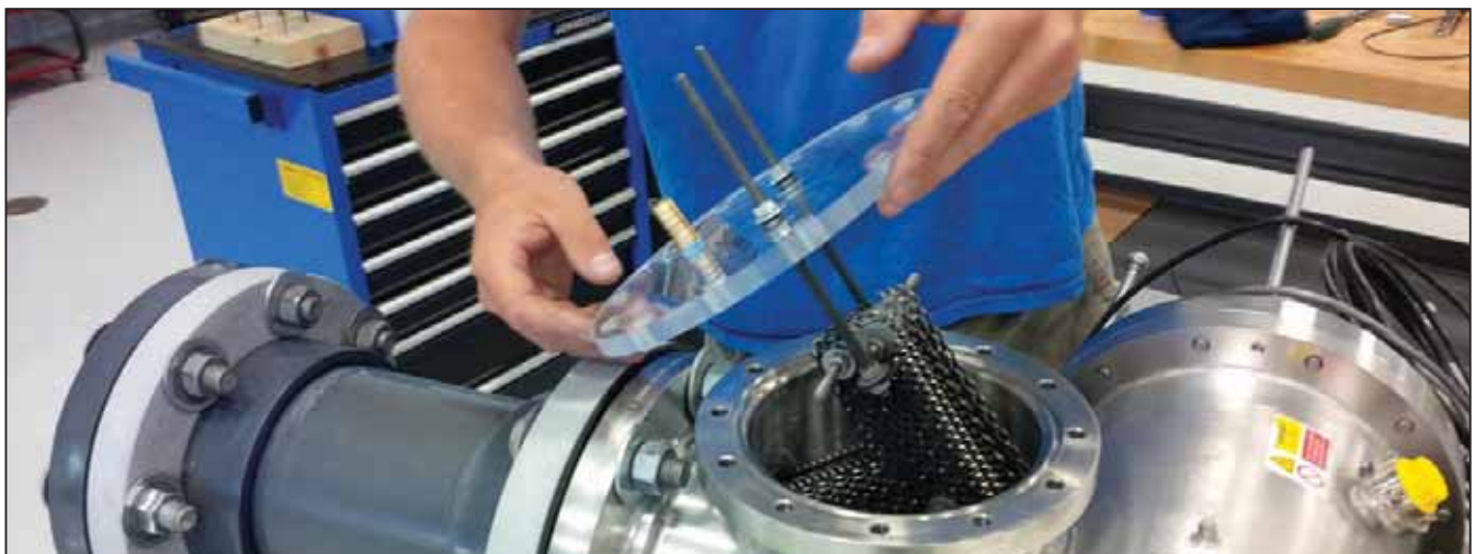
An electrode assembly is being inserted into an ETS AOP system, directly upstream of the UV lamps.
