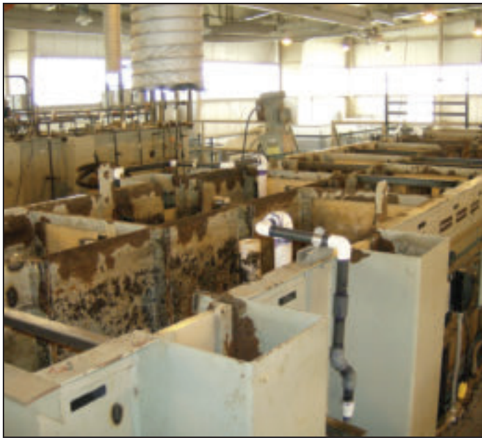
Figure 3. The Applied Research Program facility shown here supplied NYCDEP with valuable information used to shape the city’s BNR program. Sophisticated pilots were used to mimic full-scale treatment, allowing the city to gain experience with alternate modes of operation.
