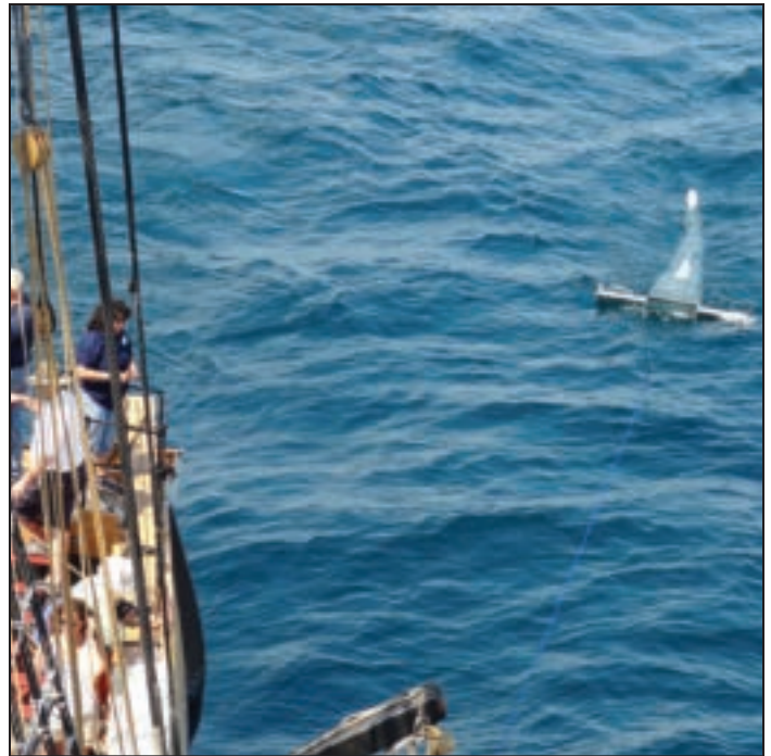
Manta trawl shown deployed during the first-ever open-water Great Lakes survey to examine plastic pollution in the Great Lakes
