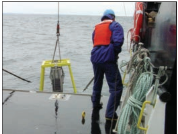
The box corer, a device for extracting sediment samples from the bottom of the lake to find contaminants, is shown being lowered.
