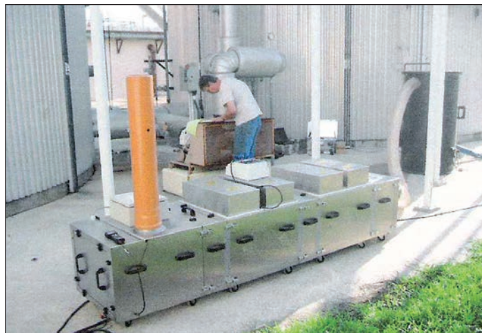
Photoionization pilot unit from Ambio Biofiltration, Ltd.
