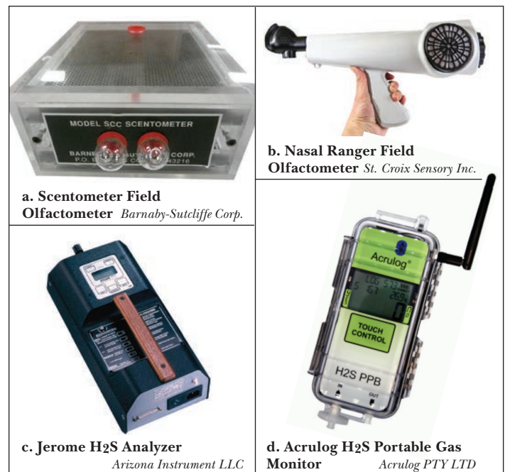
Figure 1. Odor monitoring instruments.
