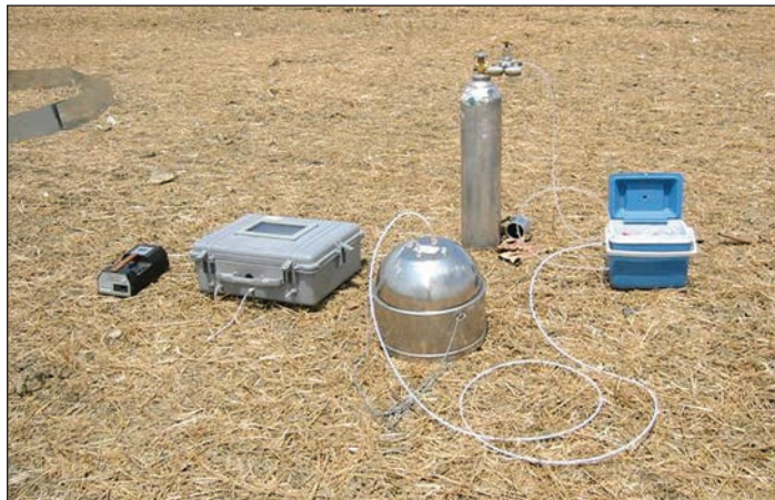
Flux chamber system used for odor sampling.
