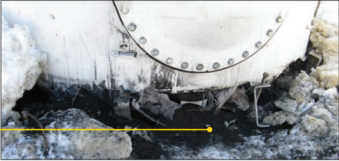
Photograph 2. Close-up of the blown-out carbon absorber. Gary Arthur
