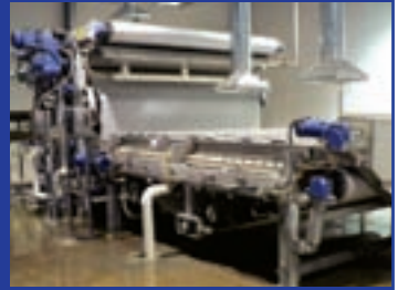
Floor Level 3.0 m model 3DP No platforms or stairs required!
