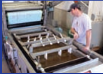
Compact 0.9 m Model DDP Belt Press Great concept for small plants.
