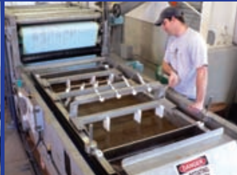
Compact 0.9 m Model DDP Belt Press Great concept for small treatment plants.
