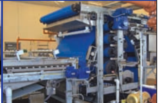
Dual Purpose 1.5 m model 3DP Operates as a Gravity Belt Thickener or Belt Press.
