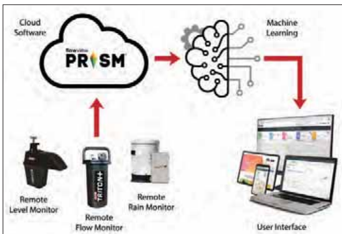
Figure 2. The remote monitors continuously measure and communicate conditions to cloud-based software. This software uses machine learning to recognize a developing blockage. The software alerts the users through interfaces when cleaning is necessary. ADS Environmental Services
