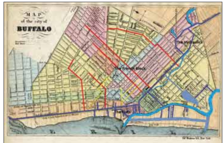
Map of The City of Buffalo, Charles Magnus lithograph, New York, circa 1850, (hand colored map on a letter sheet). Modern digital addition denotes the locations of the following: red lines are trunk sewers; yellow lines are side sewers; light blue lines are natural waterways; dark blue lines are completed canals; gray lines are canals under construction.
