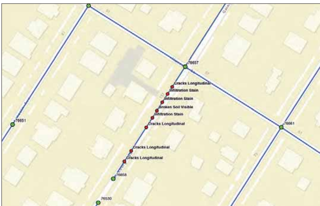
Figure 4. GIS map displaying observed CCTV condition points mapped along sanitary sewer pipe sections. GHD Consulting Services Inc.
