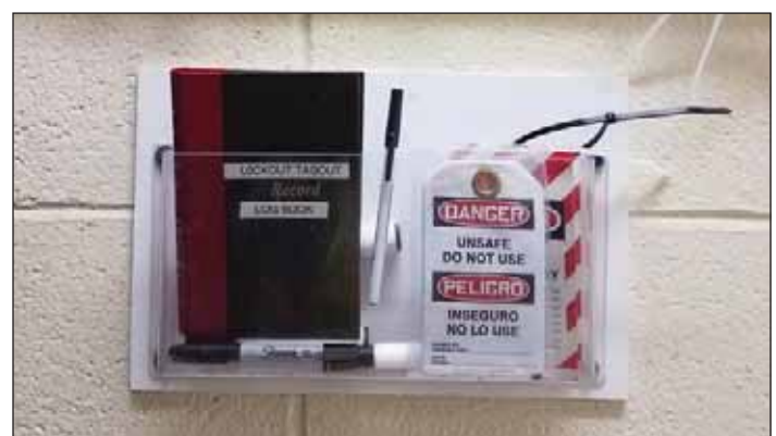
Kept below the Lock Out/Tag Out station is the Lock Out/Tag Out shift change log.
