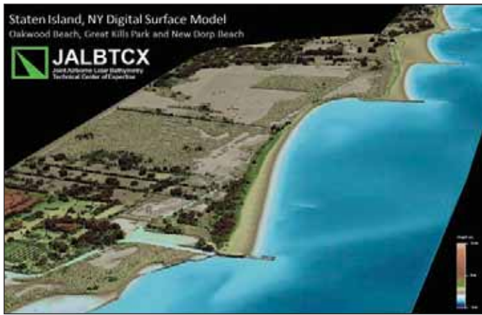
A sample of the type of elevation images the JALBTCX team developed for the U.S. Army Corps of Engineers, New York District. This image shows the shoreline elevations along the coast of Staten Island, New York. USACE
