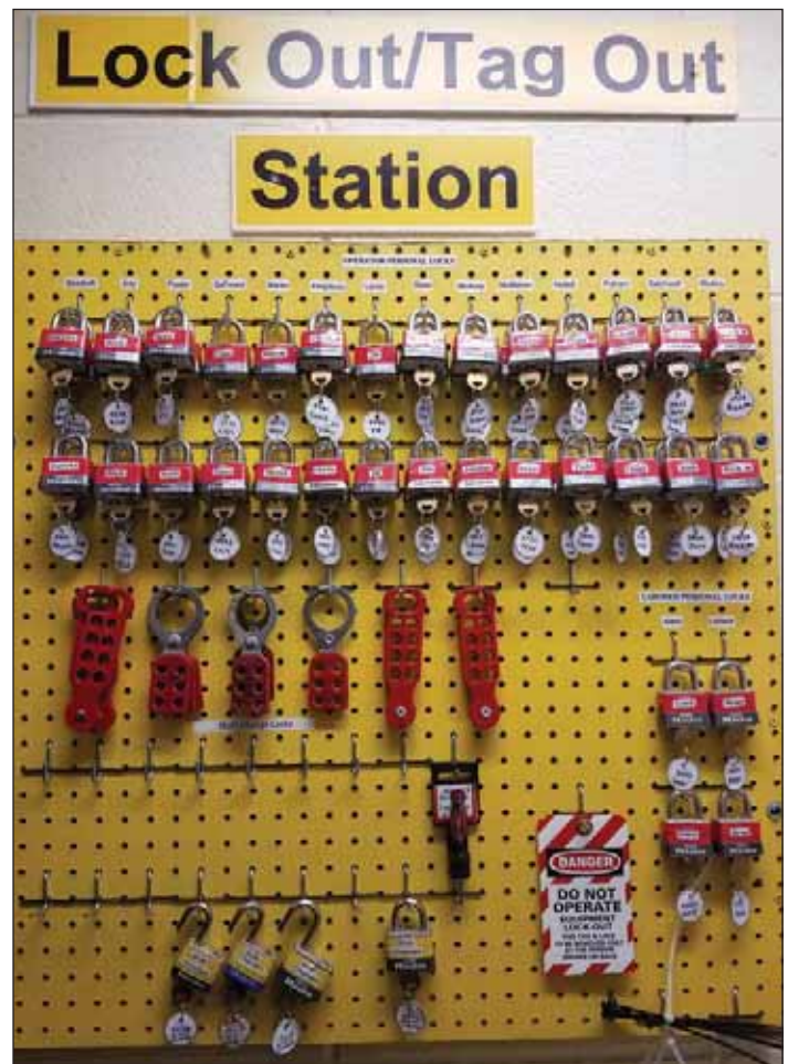
The Lock Out/Tag Out station is the central location at the facility for access to the locks and tags.
