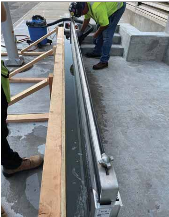
Testing of one of many flood barriers implemented under the Program. AECOM
