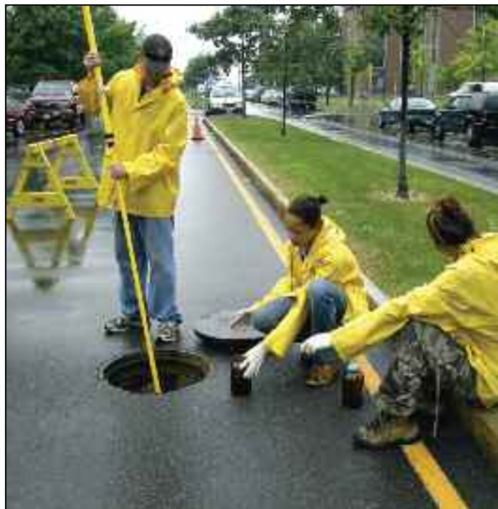
Sampling stormwater quality to assess the efficacy of a vortex separator on the Buffalo State campus
