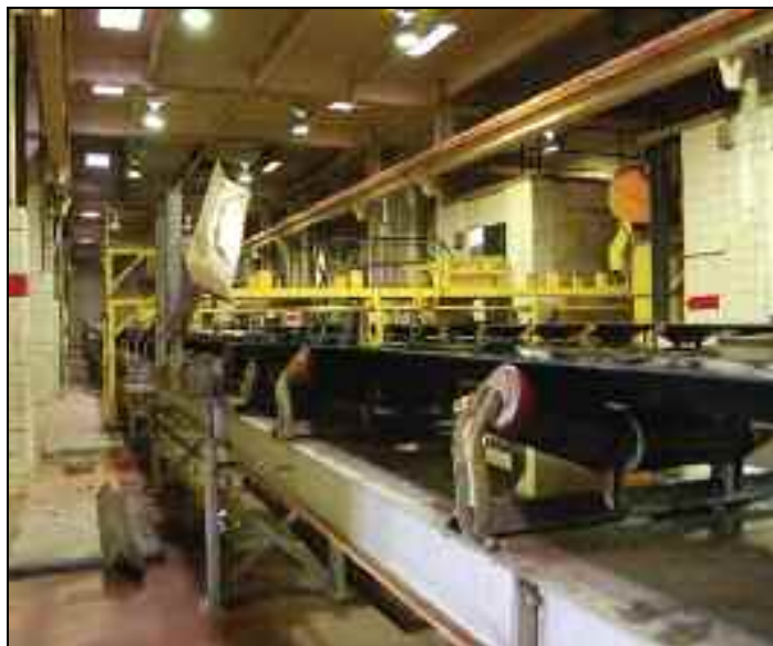
Sludge trucked to the Buffalo Sewer Authority will be distributed to this conveyor belt system at which staff will determine whether it will be processed through incineration or through the rewetting system.
