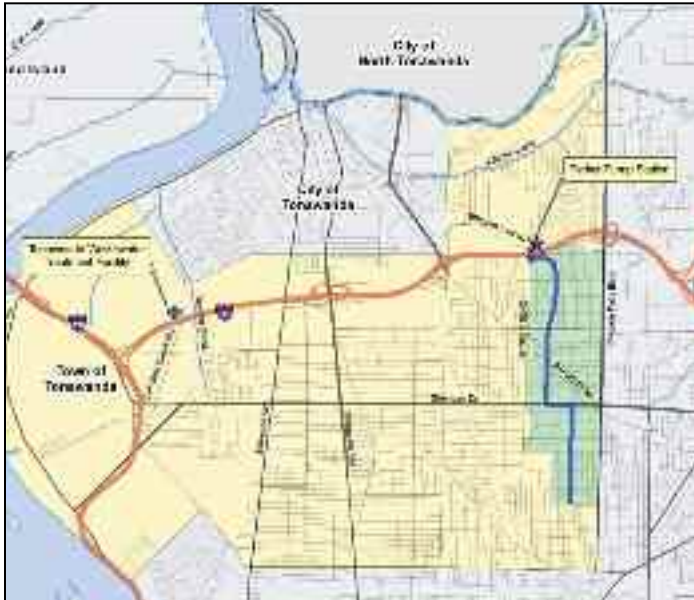
The Parker-Fries Interceptor project, which terminates at the Parker Pump Station just south of I-290, calls for key tributary interceptors and trunk sewers to be upsized.
