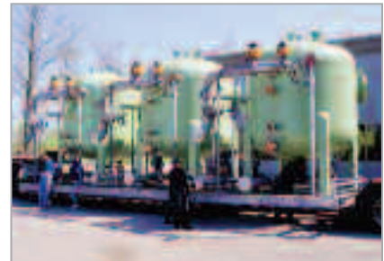
Skid Mounted Pressure Sand Filters
