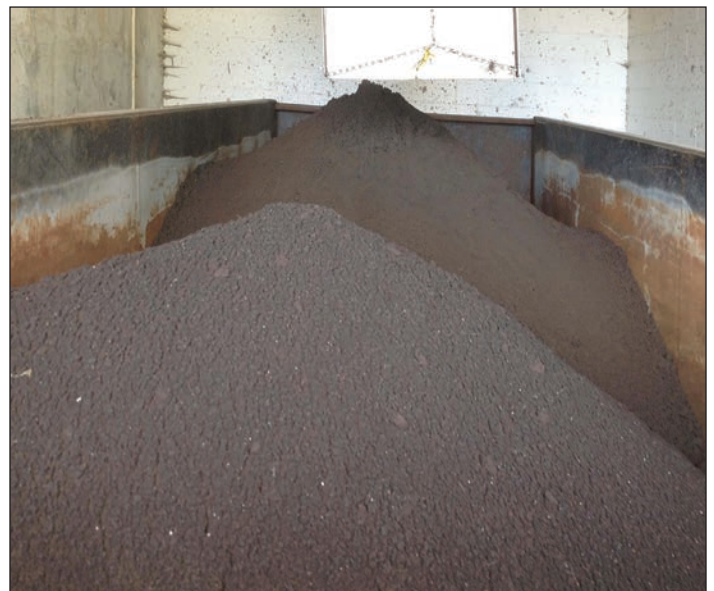
Dewatered biosolids output from the new 18-inch diameter screw press
