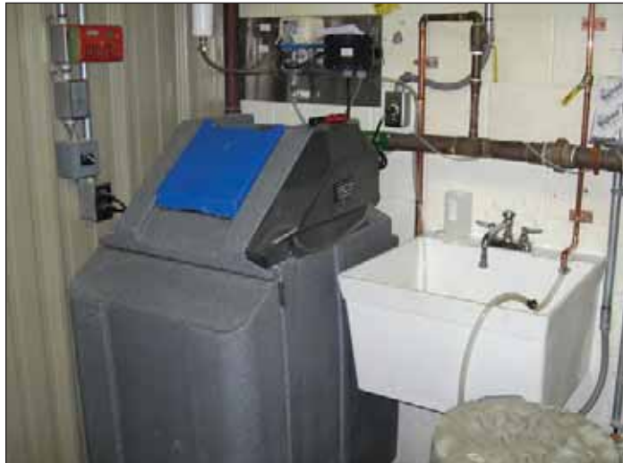
Photograph 3. The 24-hour composite sampler collects samples of SHIA's wastewater for BOD 5 analyses. Credit: OCDWEP
