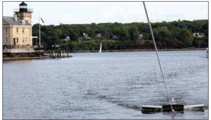
Manta trawl being towed up the tidal Rondout Creek during microplastics sampling (2014)
