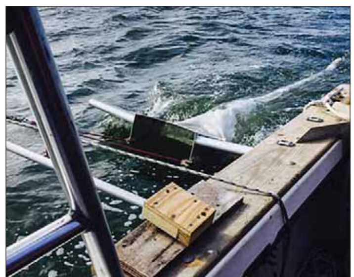
NY/NJ Baykeeper utilized a manta trawl net to gather the samples. The net is designed to float on the water's surface capturing floatable plastics.
