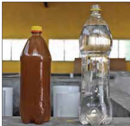
Figure 2. Raw water before AguaClara Water Treatment (left) next to potable drinking water post-AguaClara Treatment (right). This raw water is from San Nicolás, Santa Barbra, Honduras. The AguaClara treatment plant in San Nicolás provides potable water to all 6,000 people living in the municipality of San Nicolás.
