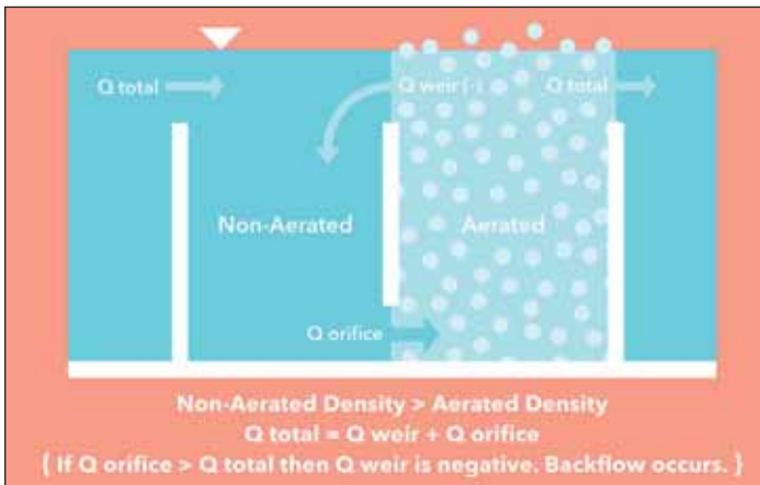
Figure 4. In some circumstances, the forward flow through the low-level orifice may exceed the forward flow rate through the tank. If that occurs, then flow will return to the upstream zone by passing back over the weir in reverse.
