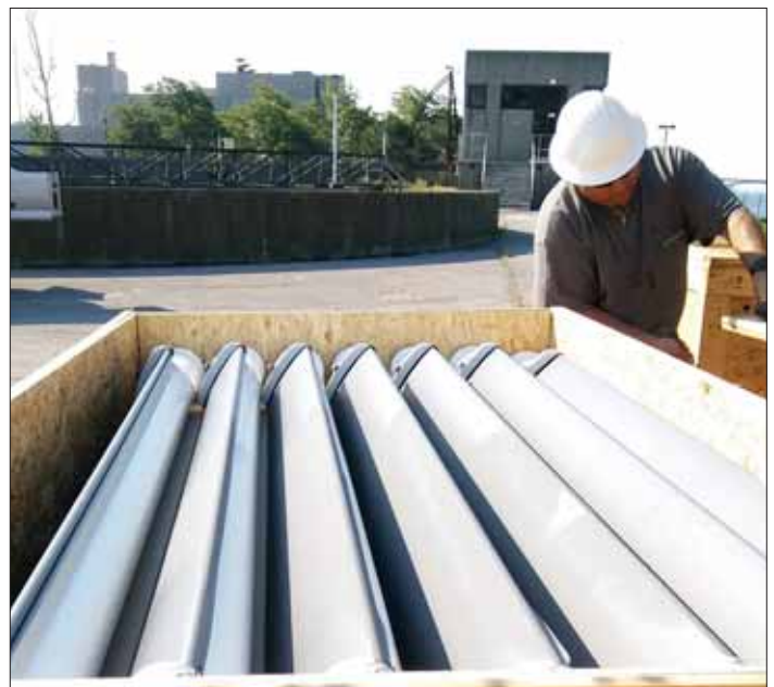
Figure 2: Sanitaire® Gold Series strip diffusers delivered to the Bird Island WRRF.
