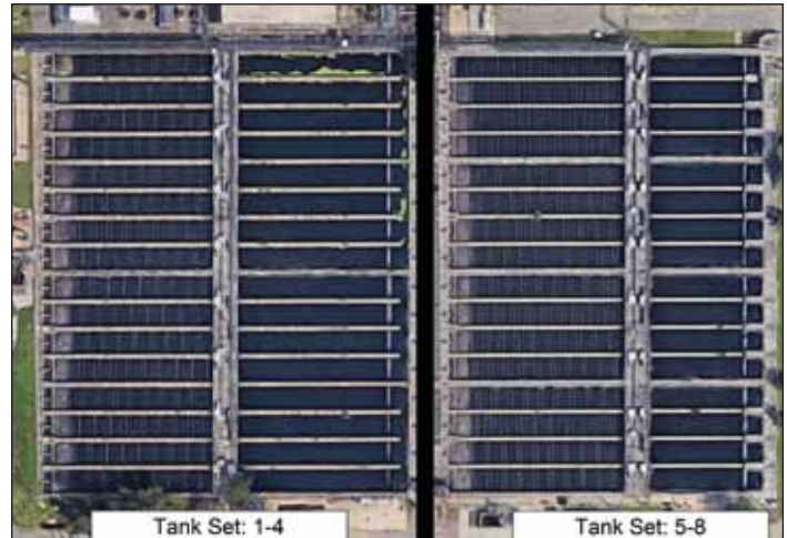
Figure 3. Plan view of clarifiers: Tanks 1 through 4 (left) and Tanks 5 through 8 (right). Google Earth
