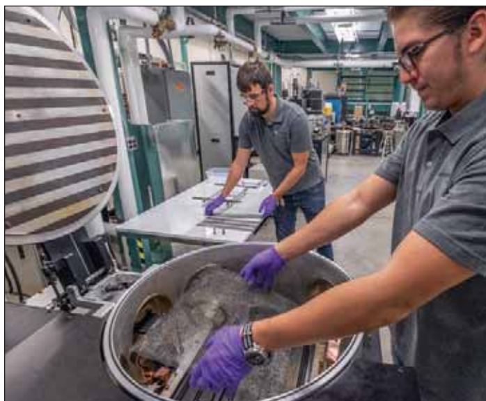
Engineers Juan Donoso (foreground) and Robert Rechenberg prepare a hot-filament diamond reactor to destroy PFAS compounds at Michigan State University's Fraunhofer Center for Coatings and Diamond Technologies on Sept. 13, 2018. Derrick L. Turner/Michigan State University.
