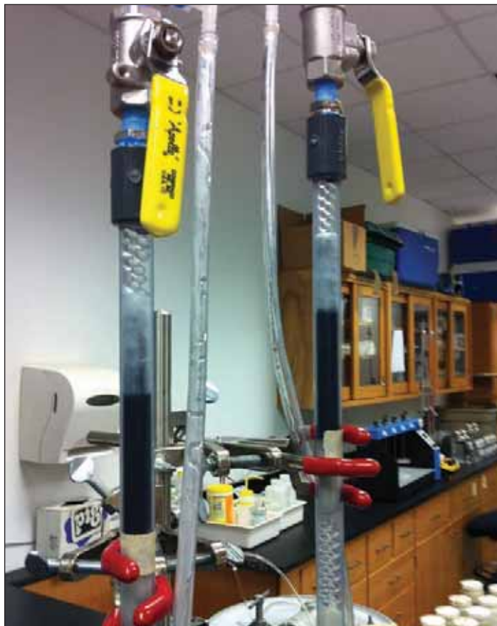
Figure 6. Figure 6. Rapid small-scale column test (RSSCT) column packing.
