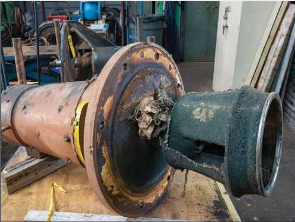
Wards Island WRRF impeller from E Battery RAS pump, damaged beyond repair, caused by wipes. Jean Schwarzwald/DEP
