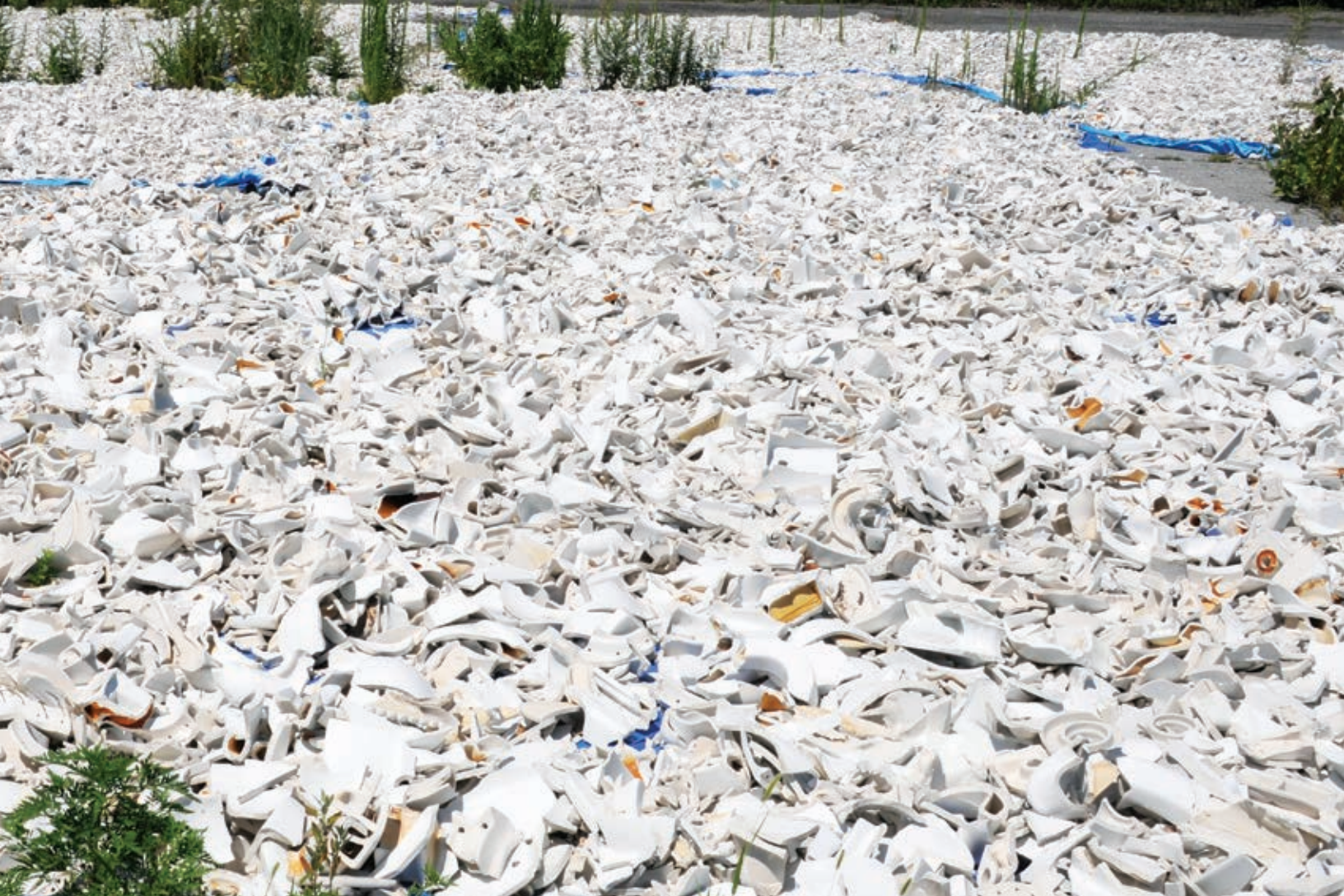
Porcelain harvested from nearly 5,000 inefficient toilets is being used to create four smaller receiving beds composed of clam/oyster shell and broken porcelain.
